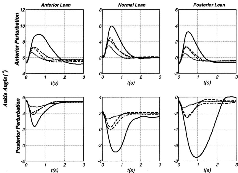
Fig. 2. Ankle angle for different experimental conditions based on averaging over ten trials for each experimental condition (subject No. 8). The onset of the disturbance is set to time 0 s. Different line styles indicate different perturbation types according to Table 1: type 1  $\Rightarrow$  dotted line, type 2  $\Rightarrow$  dash-dotted line, type 3  $\Rightarrow$  dashed line, type 4  $\Rightarrow$  solid line.
