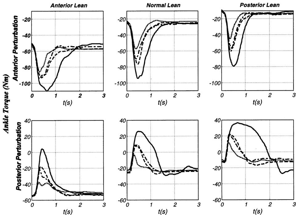
Fig. 4. Ankle torque for different experimental conditions based on averaging over ten trials for each experimental condition (subject No. 8). The onset of the disturbance is set to time 0 s. Different line styles indicate different perturbation types according to Table 1: type 1 ⇒ dotted line, type 2 ⇒ dash-dotted line, type 3 ⇒ dashed line, type 4 ⇒ solid line.
