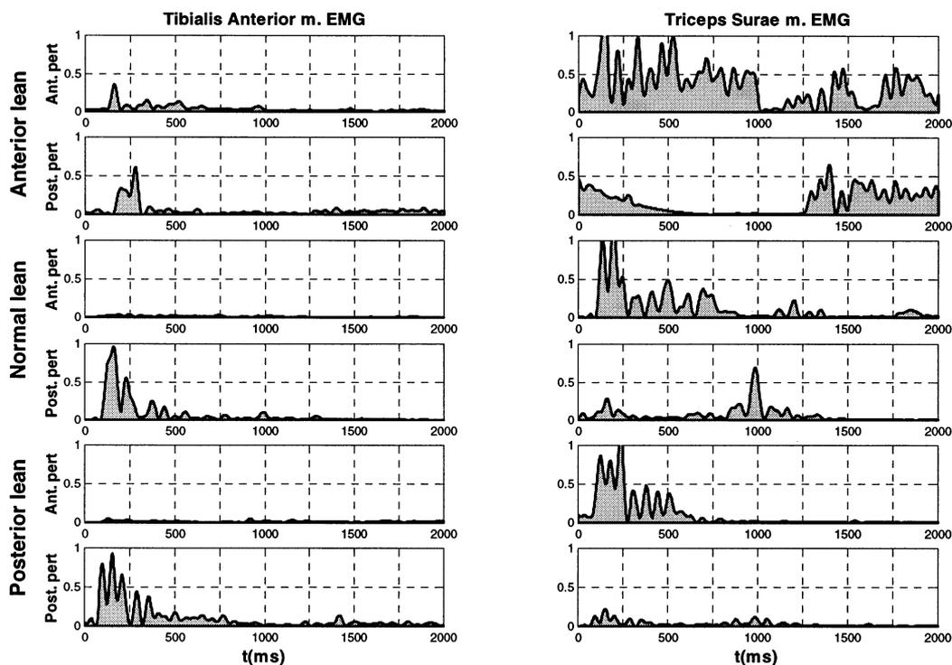
Fig. 5. Normalized characteristic time signatures of the EMG signals of tibialis anterior and triceps surae muscles for different initial stance postures and perturbation directions (subject No. 8, perturbation type 3). The onset of the disturbance is set to time 0 s.
