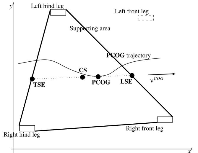
**Fig. 1.** Top view of a quadruped supporting area with left front leg in swing phase
