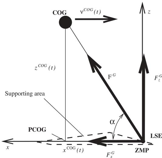
Fig. 2. Calculation of dynamic stability: planar, translation only approach
