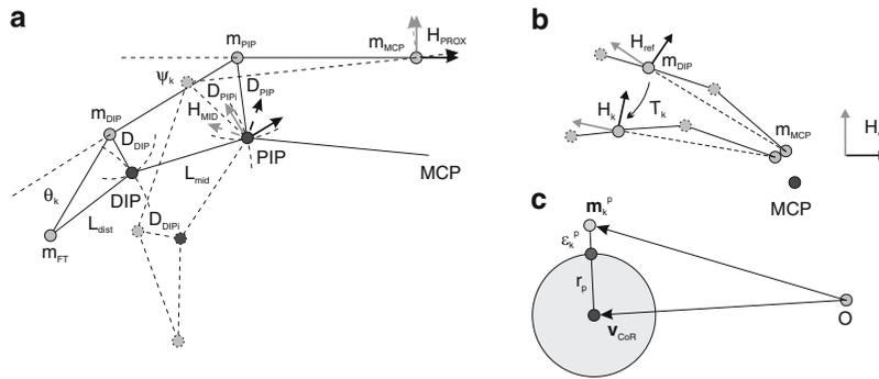
**Fig. 3** Assessment of centers of rotation of the PIP and DIP joints of fingers and the MCP and IP joints of the thumb [23] (a), MCP joints of fingers [16] (b), and CMC joint of the thumb [6] (c)
