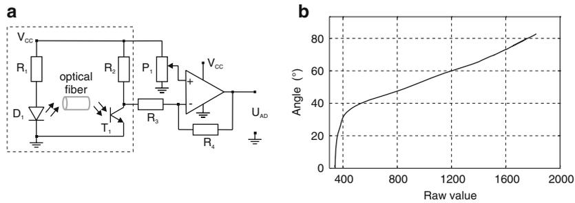
**Fig. 5** Technical implementation of an optical goniometer (a), and its sensitivity (b) recorded for the sensor mounted onto two stiff segments linked with a hinge joint
