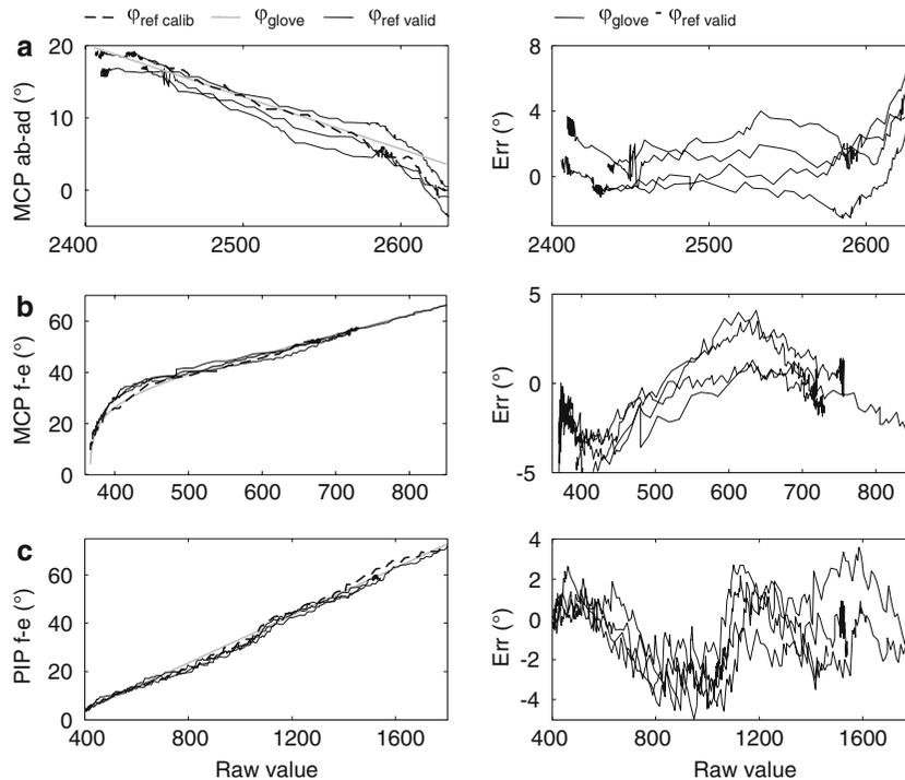
**Fig. 7** Accuracy of the glove, calibrated with the reference method ( $\varphi_{\text{ref calib}}$ ): relative ab-ad between the index and middle fingers (a), f-e of MCP (b) and PIP (c) joints of the index finger. Right panels: the difference between the reference angles ( $\varphi_{\text{ref valid}}$ ) and the angles measured with the calibrated glove ( $\varphi_{\text{glove}}$ )
