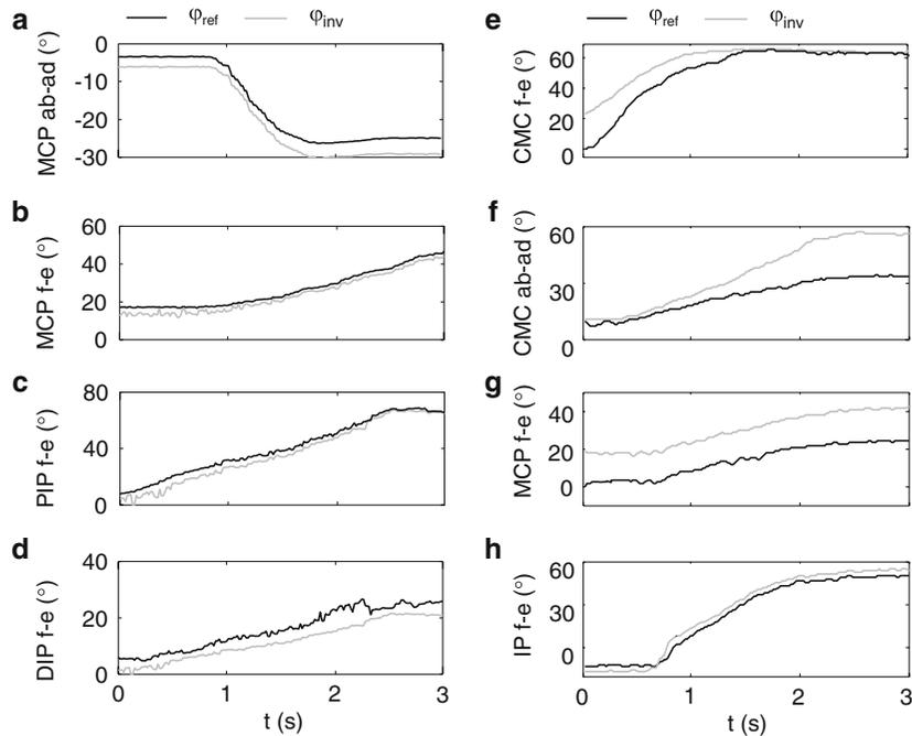
**Fig. 6** Ab-ad of MCP joint (a), f-e of MCP (b), PIP (c), and DIP (d) joints of the index finger, f-e of CMC (e), ab-ad of the CMC joint (f) and f-e of the MCP (g) and IP (h) joints of the thumb estimated from the CoR of joints (black line) and through inverse kinematics (gray line)
