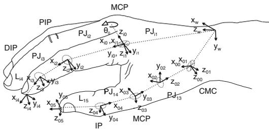
**Fig. 1** Finger joints used in a kinematic model of a finger and the thumb
