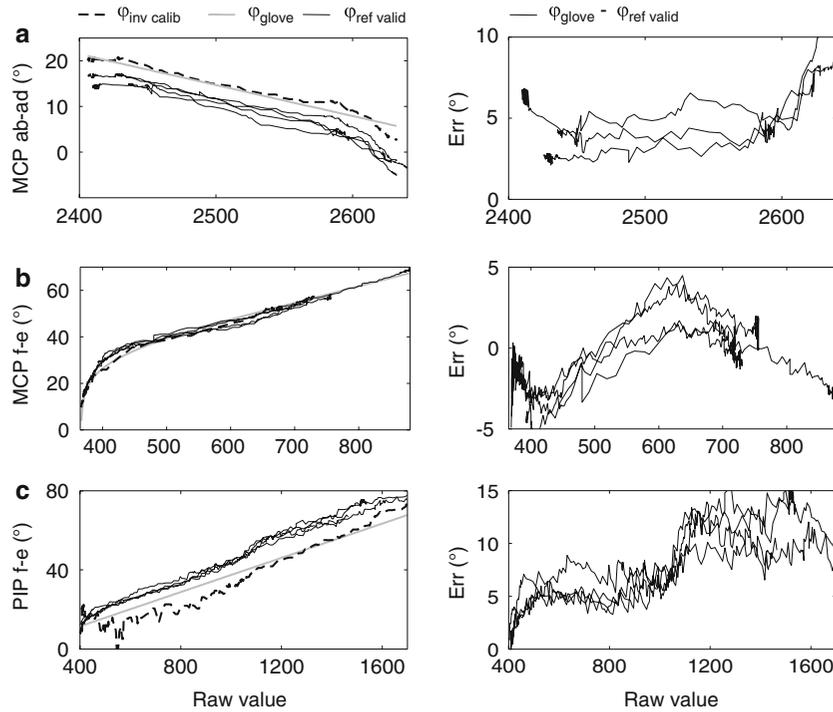
**Fig. 8** Accuracy of the glove, calibrated with the inverse-kinematics method ( $\varphi_{inv\ calib}$ ): relative ab-ad between index and middle fingers (a), f-e of MCP (b) and PIP (c) joints of the index finger. Right panels: the difference between the reference angles ( $\varphi_{ref\ valid}$ ) and the angles measured with the calibrated glove ( $\varphi_{glove}$ )
