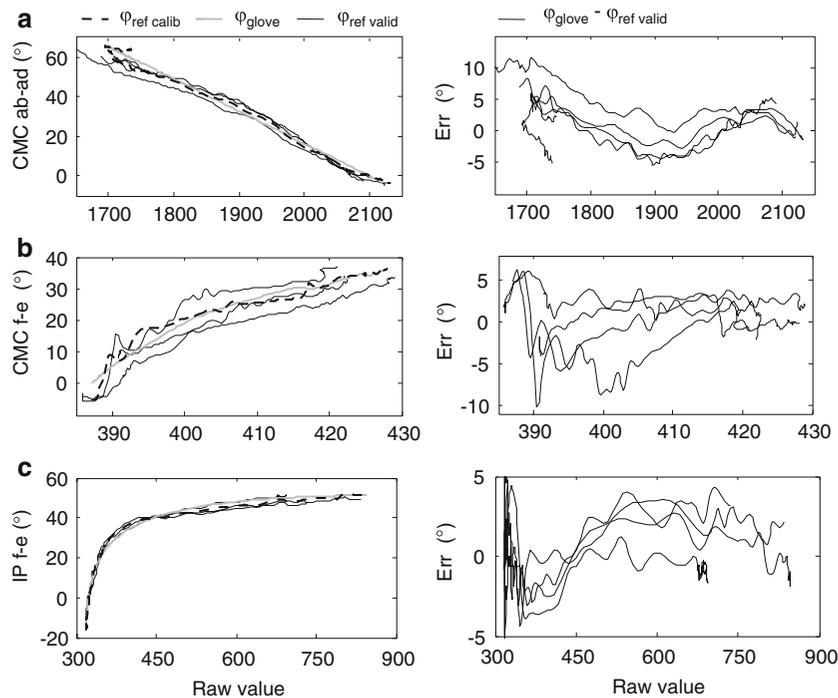
**Fig. 9** Accuracy of the glove, calibrated with the reference method ( $\varphi_{\text{ref calib}}$ ): relative ab-ad (**a**) and f-e (**b**) of the CMC joint and f-e of the IP (**c**) joint of the thumb. Right panels: the difference between the reference angles ( $\varphi_{\text{ref valid}}$ ) and the angles measured with the calibrated glove ( $\varphi_{\text{glove}}$ )
