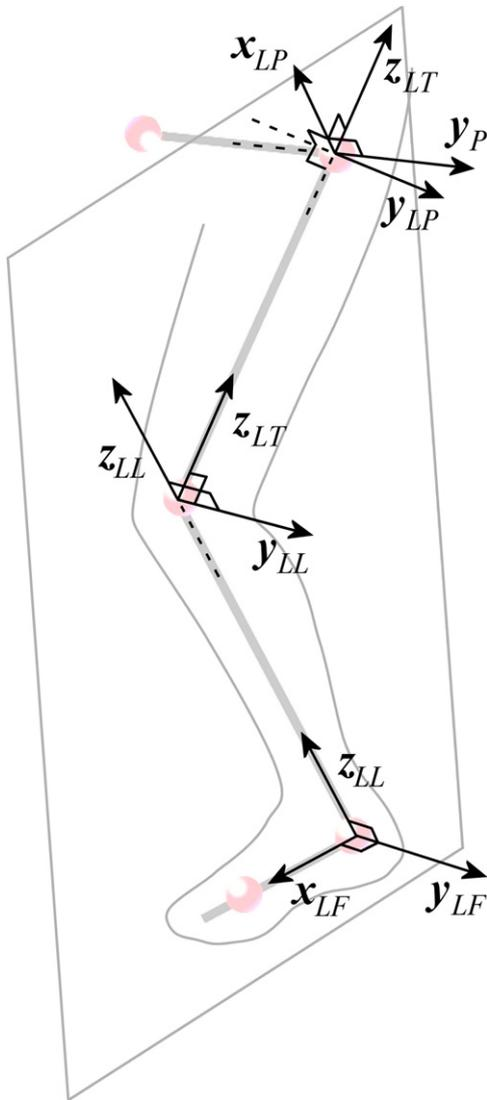
Fig. 2. Kinematic representation of the left leg showing vectors needed for knee and ankle axes computation.
