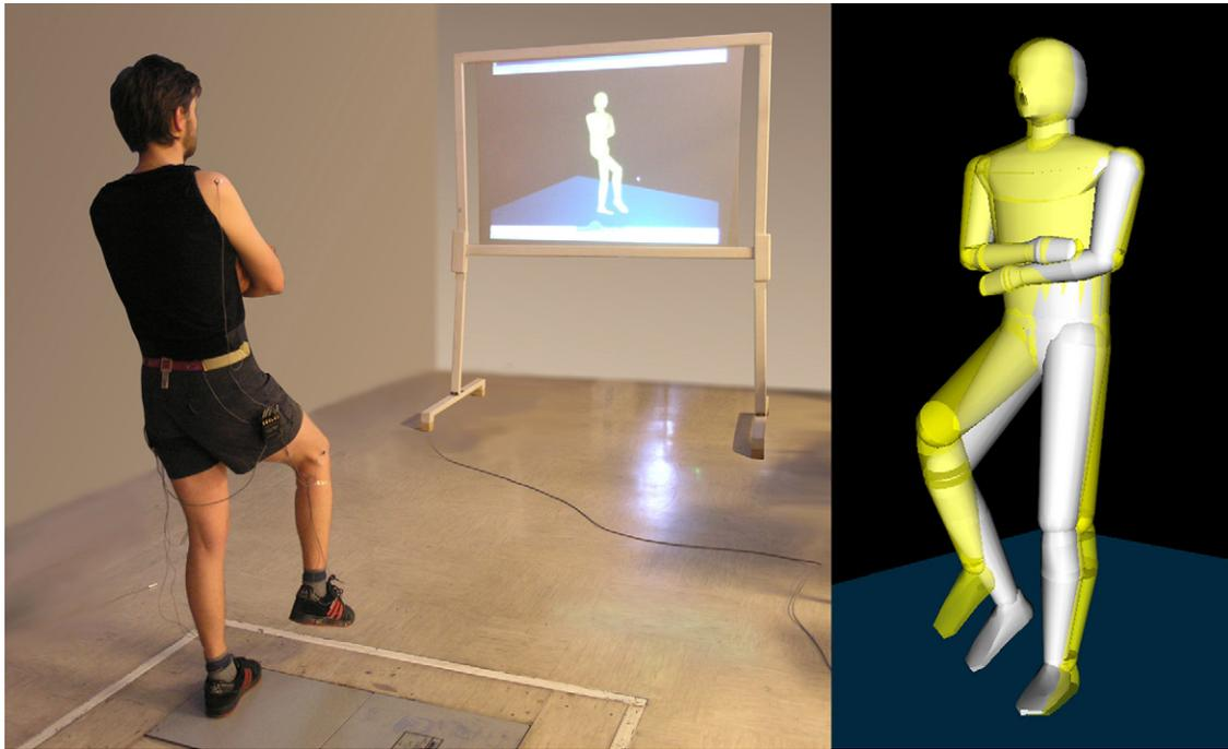
Fig. 1. Virtual mirror: a large screen showing movements of the subject in real time (left), superimposed virtual trainee and virtual instructor enlarged (right).
