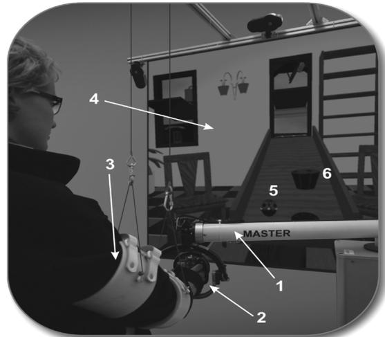
Fig. 1. A subject performing the virtual rehabilitation task. The subject performs the task using the robot (1) and grasping device (2) while his/her arm is supported by cuffs (3). The screen (4) shows a sloped table, a ball (5) and a basket (6).
