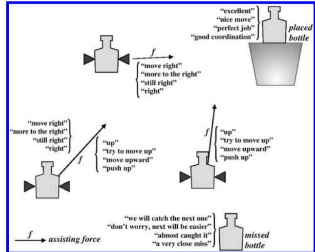
**Figure 7.** Verbal instructions, picked by an adaptive algorithm, are used for user encouragement in various stages of the movement task.
