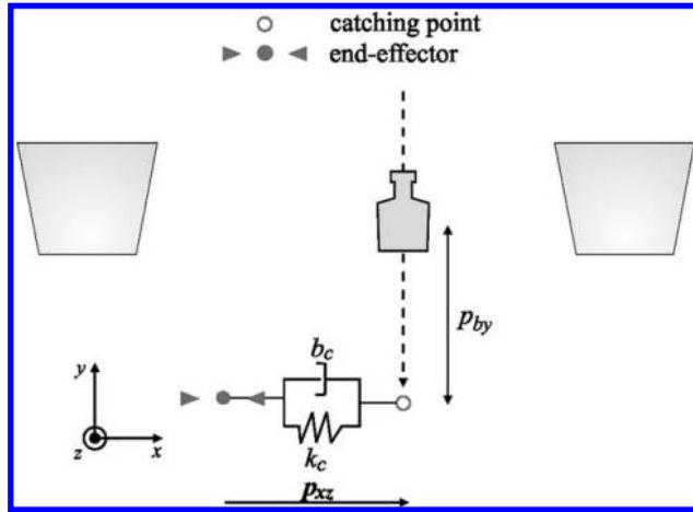
**Figure 4.** Catching assistance leads the subject in  $xz$  plane to the catching point with an impedance controller.
