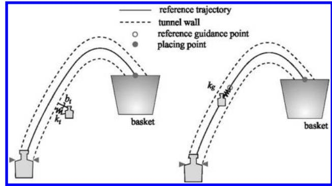
**Figure 5.** Two impedance controllers included in the tunnel assistance. The controller that allows only small deviations from the central trajectory is shown on the left side. On the right side, the guidance controller leading the subject's arm along the desired trajectory is shown.
