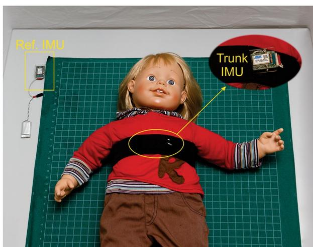
**Fig. 1** Experimental set-up, where the doll is equipped with the trunk IMU and placed in supine on the pressure mattress, while the referential IMU is placed in parallel with the pressure mattress
