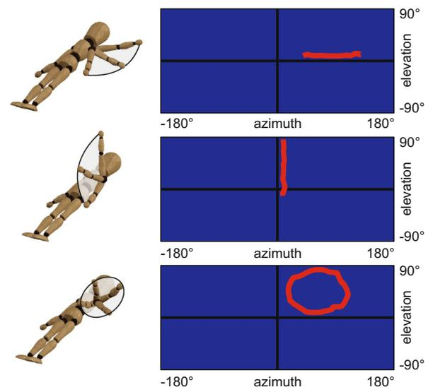
**FIGURE 2.** Representation of the FA orientation map determination for arm movements with changes of azimuth angle (top subplot), elevation angle (middle subplot), and both angles simultaneously (bottom subplot).
